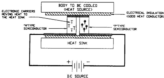
Figure 1: Cross Section of a Typical TE Couple
