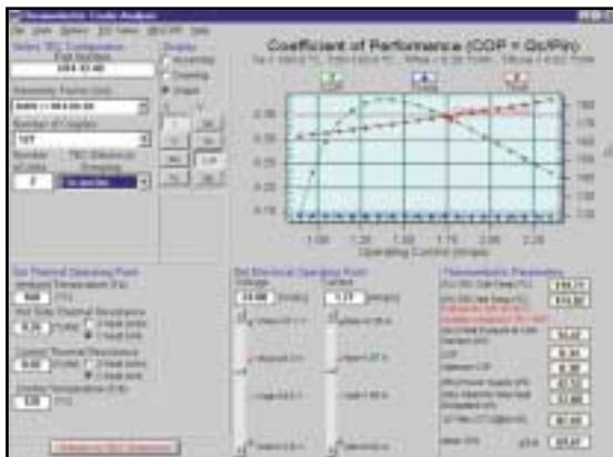
Use AZTEC to model the performance of any standard thermoelectric cooler in our inventory, using your operating conditions.
