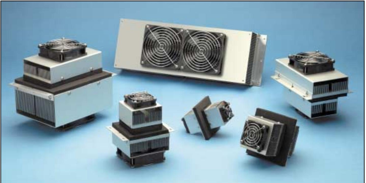
The MELCOR Thru Mount Series Thermoelectric Air Conditioners are designed for electronic cabinets, refrigeration and environmental chambers where temperature control is critical. Because there is no air exchanged between the cabinet and the ambient, these closed loop air conditioners are ideal for NEMA 12 requirements. They are virtually maintenance-free, with no filters to change, and can be moved in any orientation, offering design flexibility with solid-state reliability.
