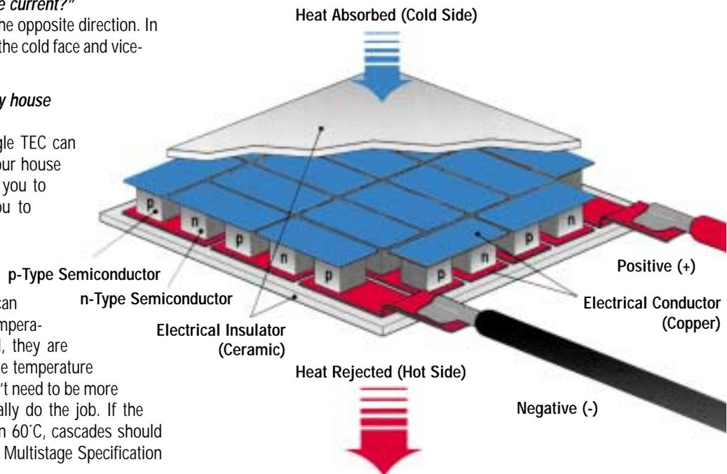
*Cutaway drawing shows the construction of a single-stage TEC. During operation, DC current flows through the p- and n-type couples causing heat to move from the cold side to the hot side of the TEC. In many applications, some type of heat exchanger will be used on the hot side of the TEC to move heat away from the unit.*
