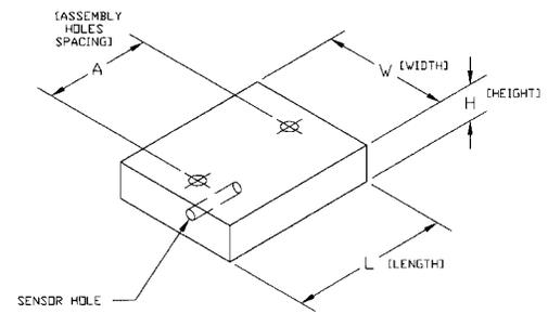
MELCOR's spacer blocks widen the gap between the cold surfaces and hot side heat exchanger, allowing for more insulation material. The spacer blocks are intended for use with our CP, PT, or HT series of thermoelectrics as part of a complete thermoelectric system.
